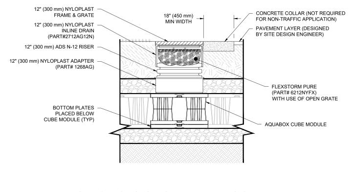
AQUABOX INSPECTION PORT INLET W/FLEXSTORM DETAIL NTS
