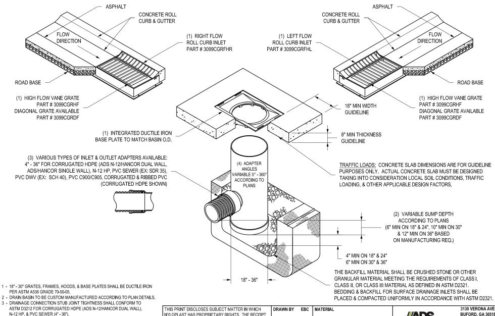
ADAPTERS CAN BE MOUNTED ON ANY ANGLE 0° TO 360°. TO DETERMINE MINIMUM ANGLE BETWEEN ADAPTERS SEE DRAWING NO. 7001-110-012.
