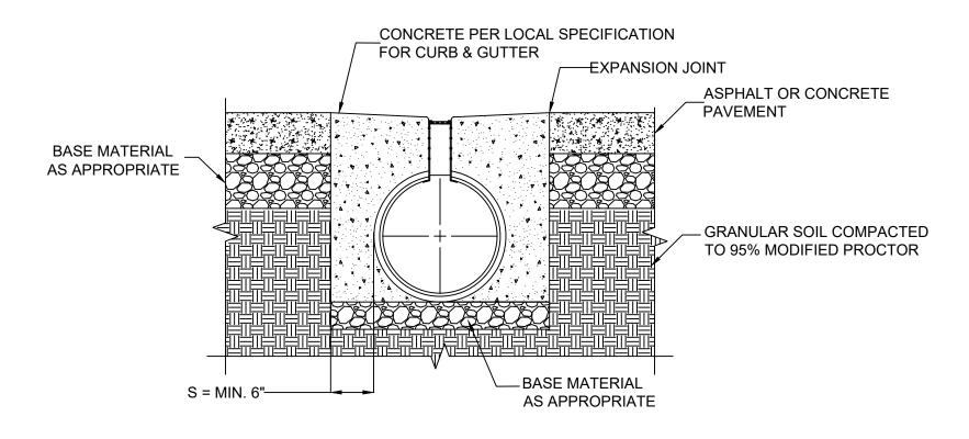
Heavy Traffic - surrounded by concrete for critical loading applications. This would include frequent high-speed, H-20 traffic (i.e. highways, loading docks, etc.). The 'S' dimension is generally 6" depending on the specific conditions for the project (design layout, traffic patterns, soil properties, etc.). Expansion joints and concrete and/or asphalt pavement is to be designed by others.
